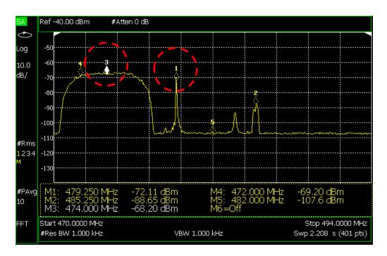
Observe the difference between maximum amplitude of the video carrier of the TV signal (1) and the max amplitude of WSD (3)
